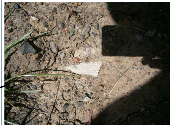
Photo 4: Potential ACM fragment close-up
